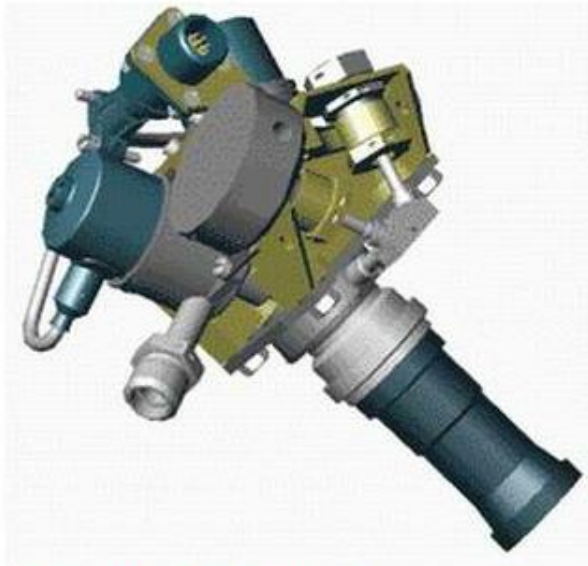
Cyclone-3 LV thruster of 30 N thrust
